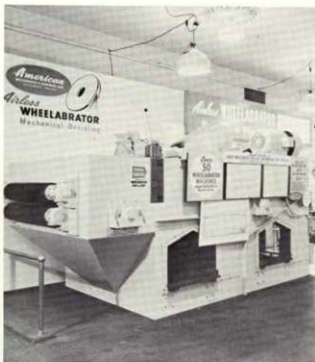
One section of Wheelabrator mechanical descaler for continuously hot rolled carbon steel strip. Actual size of this special machine is more than four times as large as section shown here.
